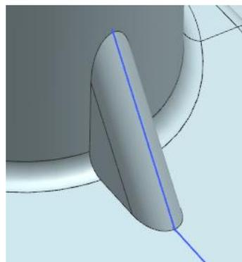
The next step consists in adding a fillet around the edge of the stiffener
